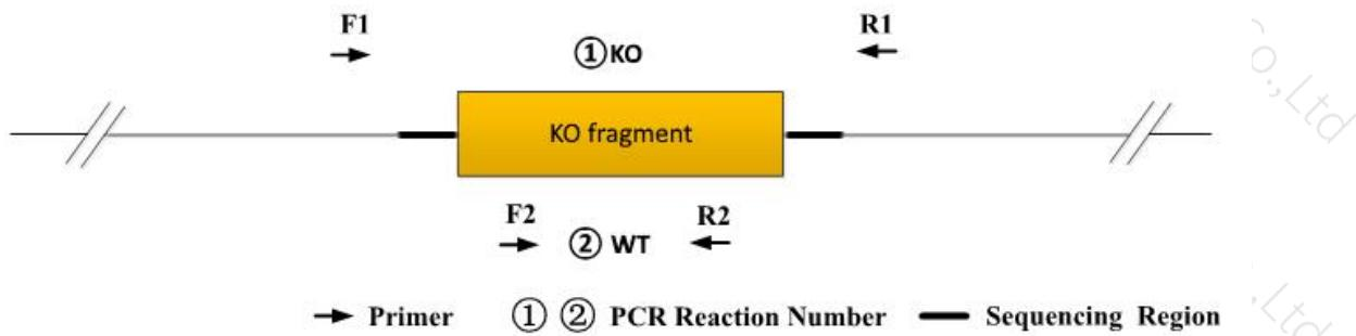
Wild type: ①PCR reaction obtains a single WT band; ②PCR reaction obtains a single WT band.
