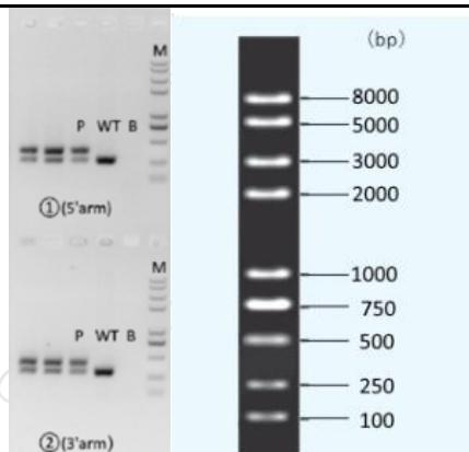
Note: P: Heterozygous samples; WT: Wildtype control; B: Blank control (ddH<sub>2</sub>O); M: DNA Ladder
